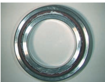
Photo. 6.1 Filling grease into angular contact ball bearing
