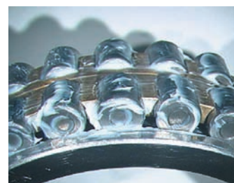
Photo. 6.2 Filling grease into cylindrical roller bearing
