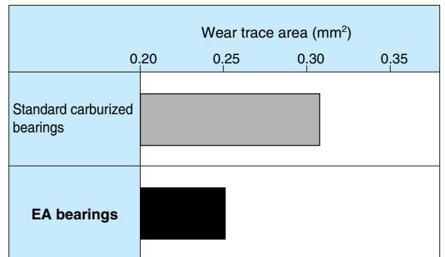
Fig.9 Results of fretting wear test
