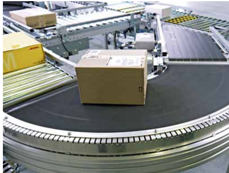
Curved conveyor in a distribution centre.
