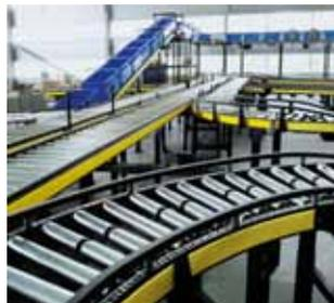
**Siegling Extremultus Live Roller Belts** are energy-saving, durable drive components that ensure quick and reliable distribution.
