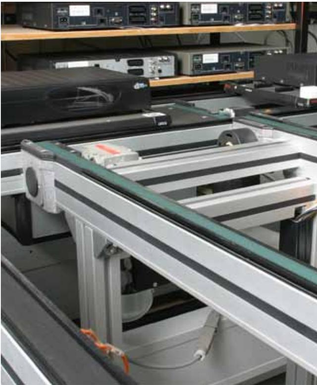
**Siegling Extremultus Drag Belts** are special developments with superior mechanical and electrostatic characteristics which make conveying and handling electronic components more efficient and safe:
