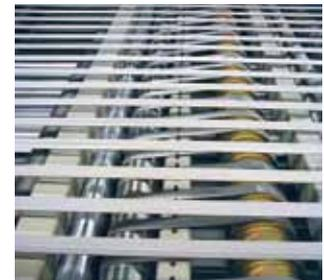
**Siegling Extremultus Machine Tapes** are vital components of machinery in many industrial applications. Tension members made of polyester fabric, polyamide sheet or elastic polyurethane which make them ideal for a wide range of applications.
